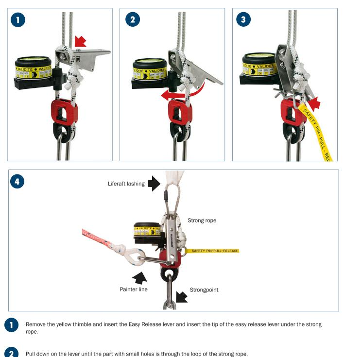
Pull down on the lever until the part with small holes is through the loop of the strong rope.
